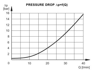
Pressure drop with free flow  $B \rightarrow A$  through check valve.
