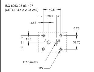
**NOTE**: The RPCED1 mounting interface, with ISO 6263 (CETOP 03) holes, must not have P and T ports or must have the 0113388 subplate (to be ordered separately)
