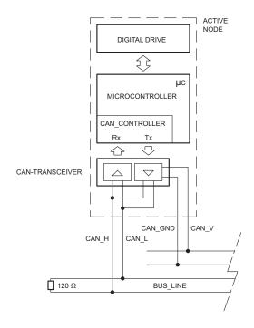
**NOTE**: If the valve is the closing node of the CAN web, insert a 120  $\Omega$  resistance on the connector pins n° 4 and 5.
