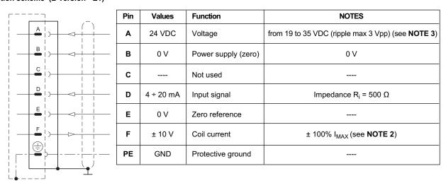
**NOTE 1**: The input signal is differential type on E0 version only. For double solenoid valves, with positive reference signal connected to pin D, the valve opening is P - A and B - T. With zero reference signal the valve is in central position. For "SA" single solenoid valves, with positive reference to pin D, the valve opening is P-B and A-T. The spool stroke is proportional to  $U_D - U_E$ .
