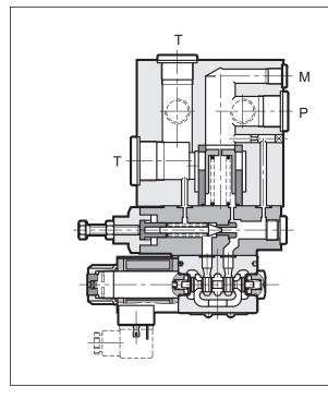
The P4D-RQM5 is a compact group that includes a pressure relief valve and it is used as mounting surface for P2D and P4D subplates.
