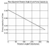
The values indicated above are at maximum pump discharge volume with the flow volume adjusting screw at the  $0^{\circ}$  position.
