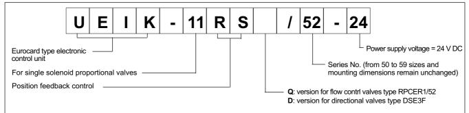
The UEIK-11RS\*/52 card is an electronic control unit Eurocard type for closed loop control of single solenoid proportional valves with positional feedback control.
