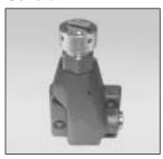
The single stage compensator consists of a spool, spring and adjusting screw, which are assembled in a body and bolted to the pump body. To control the pressure at the control piston, the spool is designed to meter flow fluid
