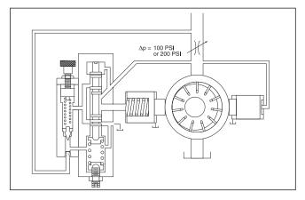
Load Sense Flow Compensator (LSFC).
