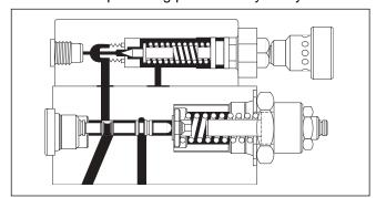
Two-Stage Compensator Cut-Away View.
