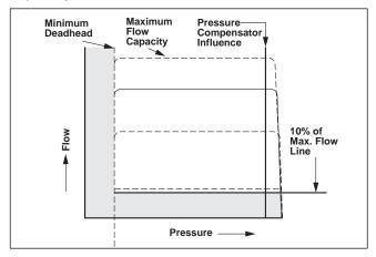
Flow Versus Pressure Characteristic Curve.
