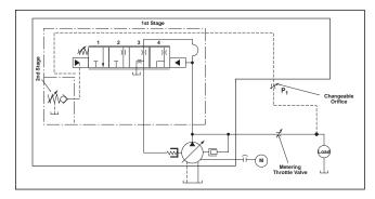
Load Sensing Flow Compensator Schematic.
