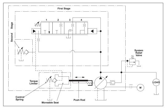
Torque Limiter Schematic.
