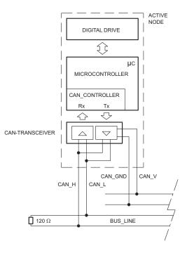
NOTE: insert a 120 Ω resistance on pin 4 and pin 5 of the CAN connector when the valve is the closure knot of the CAN network.
