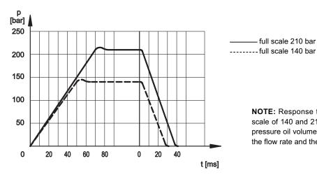
3 - RESPONSE TIMES (obtained with mineral oil with viscosity of 36 cSt at 50°C and with digital integrated electronics)
