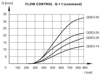
Typical flow rate characteristics  $A \rightarrow B$  for controlled flow rate: 14 - 20 - 30 - 40 l/min in function of the current supplied to the solenoid (D24 version, maximum current 860 mA, PWM 100 Hz)
