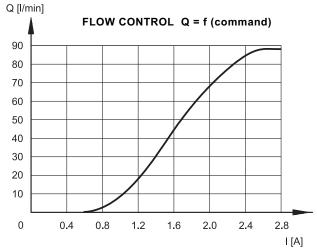
Typical flow rate characteristics A  $\rightarrow$  B in function of the current supplied to the solenoid (D12 version, max current 2.8 A, PWM 100 Hz).
