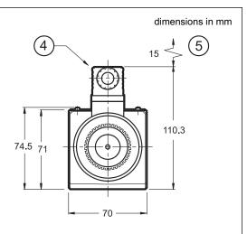
Fastening bolts: N. 4 SHC screws ISO 4762 M6x40 Torque: 8 Nm - A8.8 screws
