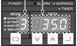
(1) Operation mode display: Displays the operation mode.
