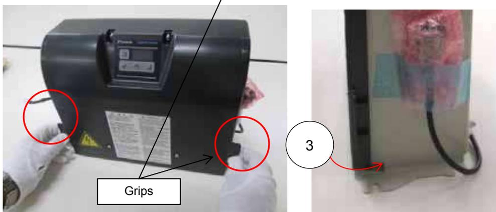
④ Press in the vicinity of the two screws at the bottom of the exterior cover to position it.
