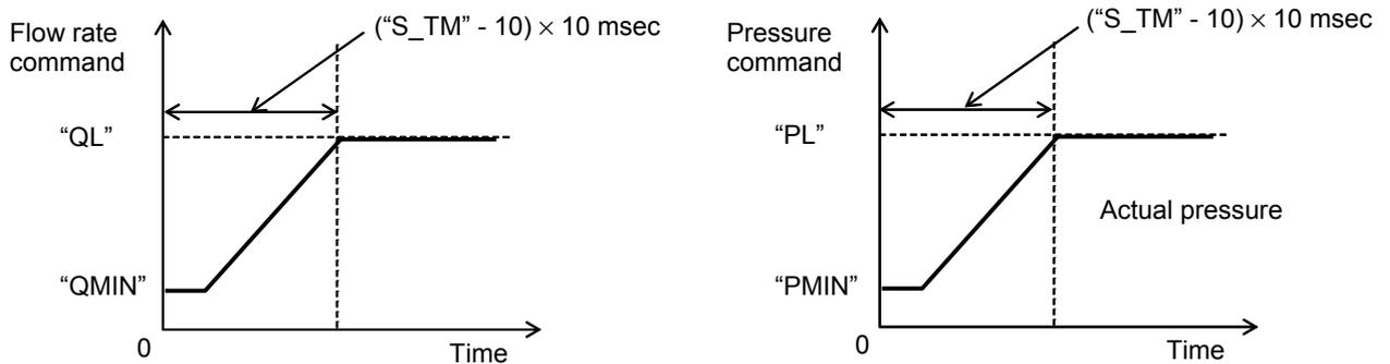
Note that the gradient of the command value can be adjusted with "S\_TM", but that the gradient is subject to restriction internally in the controller due to constraints on the response characteristics of the motor control.
