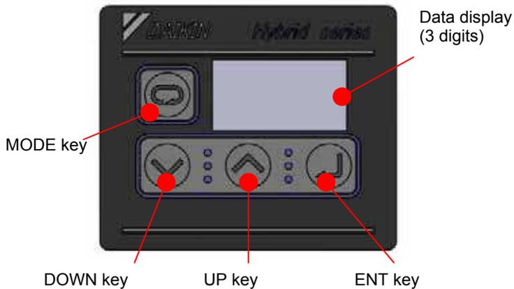
The controller features the 3-digit data display and four key-switches indicated in the figure to the left. The LED display normally shows the current actual pressure (MPa).
