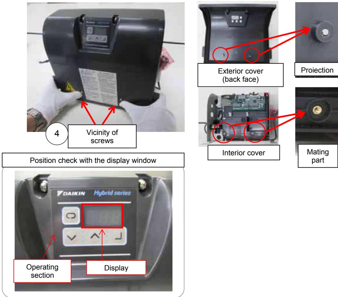
\* Check that the 7-segment display is located in the center of the display window in the operating section sheet.
