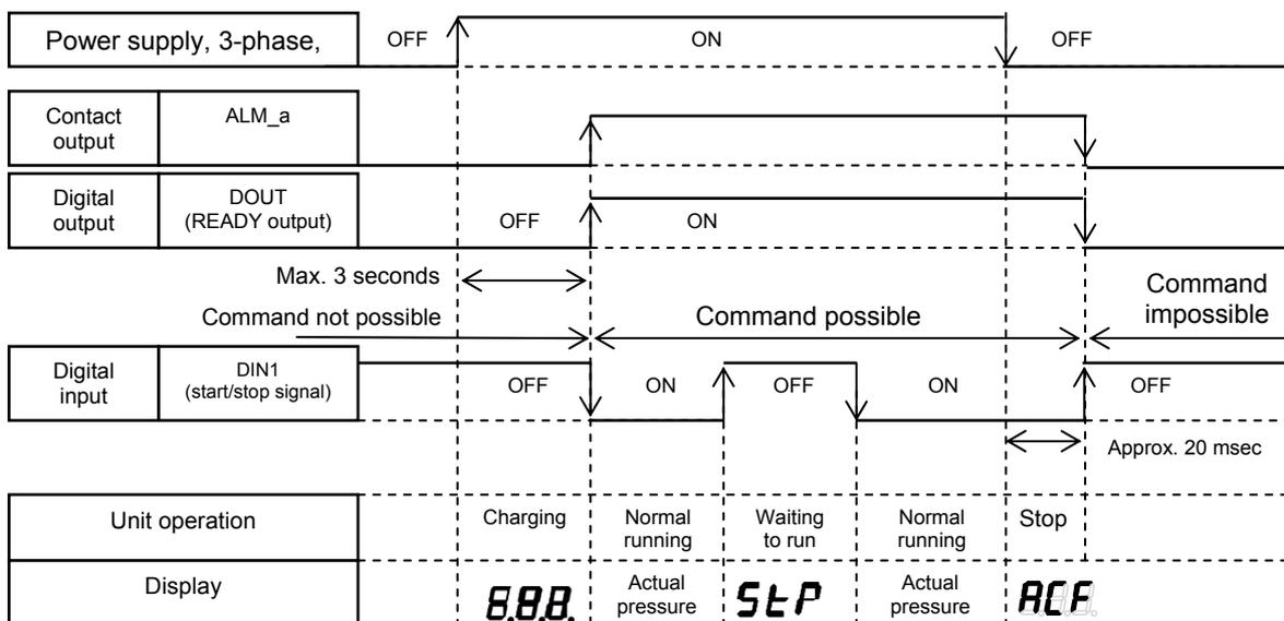
■ **Separate power supply source to control circuit**
