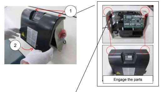
③ Holding the grips at the left and right of the cover, engage the cover with the bottom of the controller.
