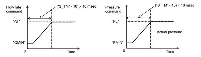
Note that the gradient of the command value can be adjusted with "S\_TM", but that the gradient is subject to restriction internally in the controller due to constraints on the response characteristics of the motor control.
