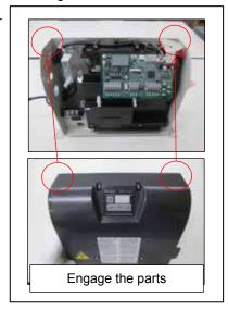
③ Holding the grips at the left and right of the cover, engage the cover with the bottom of the controller.
