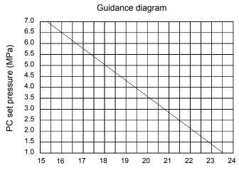
Pressure adjustment screw length (mm)
