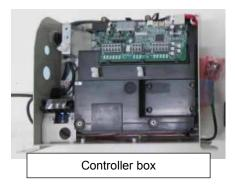
① Engage the corners of the controller and corners of the cover together and ② close the cover.
