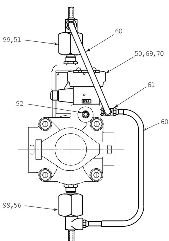
**Code 8** Rate Control Valve for Dual Pressure
