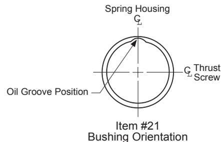
3. After the bushings are in place, check to see that the rotor shaft will fit into the bushings and provide a smooth turning fit. If the shaft turns hard, the bushings should be removed and the bore checked closely for nicks or burrs before pressing in the new bushings.
