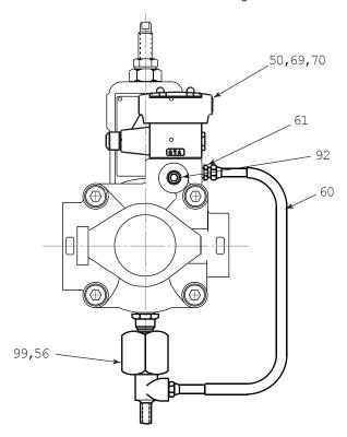
Code 8 Rate Control Valve for Dual PressureCode 9 Rate Control Valve for Dual Volume
