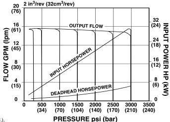
Data plotted: With oil at  $120^{\circ}$  F.  $(49^{\circ}$  C.). Viscosity @  $120^{\circ}$  F.  $(49^{\circ}$  C.) = 140 SUS.
