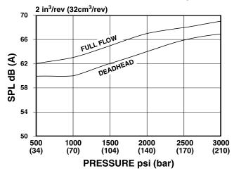
Sound pressure levels measured in a hemi-anchoic chamber with microphone placed one (1) meter
